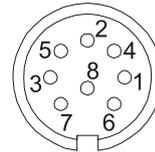
The view of the soldered side of the connector connector corresponds to the view of the pin arrangement on the encoder.
