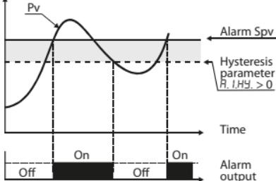
Absolute alarm with controller in heating functioning (par. 11  $R_{cL.E.}$  selected  $HER_E$ ) and hysteresis value greater than "0" (par. 28  $R_{.I.HY.} > 0$ ).
