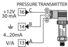
For signals 0/4....20 mA with **three-wire sensor**.
