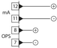
Pins 11-12: linear output in mA configurable using parameters as command (Parameter *c.outb*) or retransmission of process or setpoint (Parameter *rEtr*).
