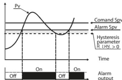
Upper deviation alarm value of alarm setpoint less than "0" and hysteresis value greater than "0" (par. 28  $R.I.HY > 0$ ).
