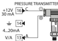
For signals 0/4....20 mA with **two-wire sensor**.
