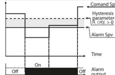
Absolute alarm refers to the command set, with the controller in heating functioning (par. 11  $R_{cL.E.}$  selected  $HER_E$ ) and hysteresis value greater than "0" (par. 28  $R_{.I.HY.} > 0$ ).
