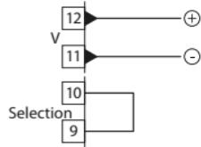
Linear output in Volt configurable using parameters as command (Parameter *c.outb*) or retransmission of process or setpoint (Parameter *rEtr*).
