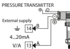
For signals 0/4....20 mA with **external power of sensor**.
