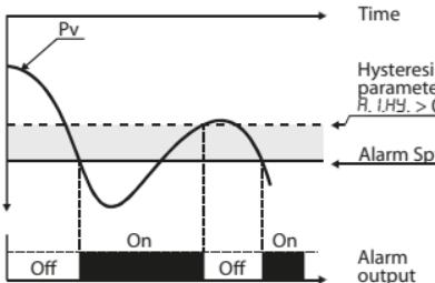
Absolute alarm with controller in cooling functioning (par. 11  $R_{cL.E.}$  selected  $Cool$ ) and hysteresis value than "0" (par. 28  $R_{.I.HY.} > 0$ ).
