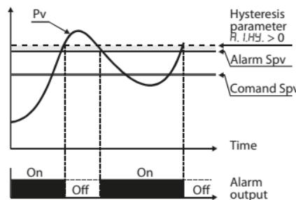
Lower deviation alarm value of alarm setpoint less than "0" and hysteresis value greater than "0" (par. 28 H.I.HY. > 0).
