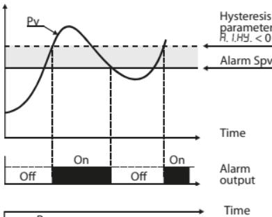
Absolute alarm with controller in heating functioning (par. 11  $R_{cL.E.}$  selected  $HER_E$ ) and hysteresis value less than "0" (par. 28  $R_{.I.HY.} < 0$ ).
