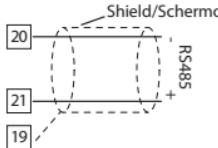
RS485 Modbus RTU communication.
