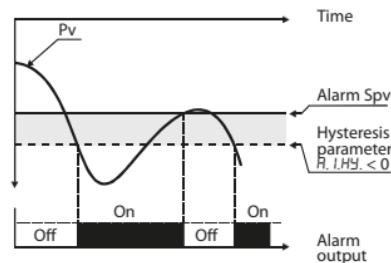
Absolute alarm with controller in cooling functioning (par. 11  $R_{cL.E.}$  selected  $Cool$ ) and hysteresis value less than "0" (par. 28  $R_{.I.HY.} < 0$ ).
